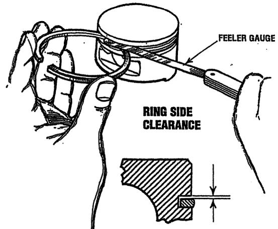
Check the clearance between the piston ring and the ring groove, if it exceeds the limit, replace the rings, the piston or both.
