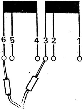
TEST EACH OF THE WINDING LEADS INDIVIDUALLY AS SHOWN
