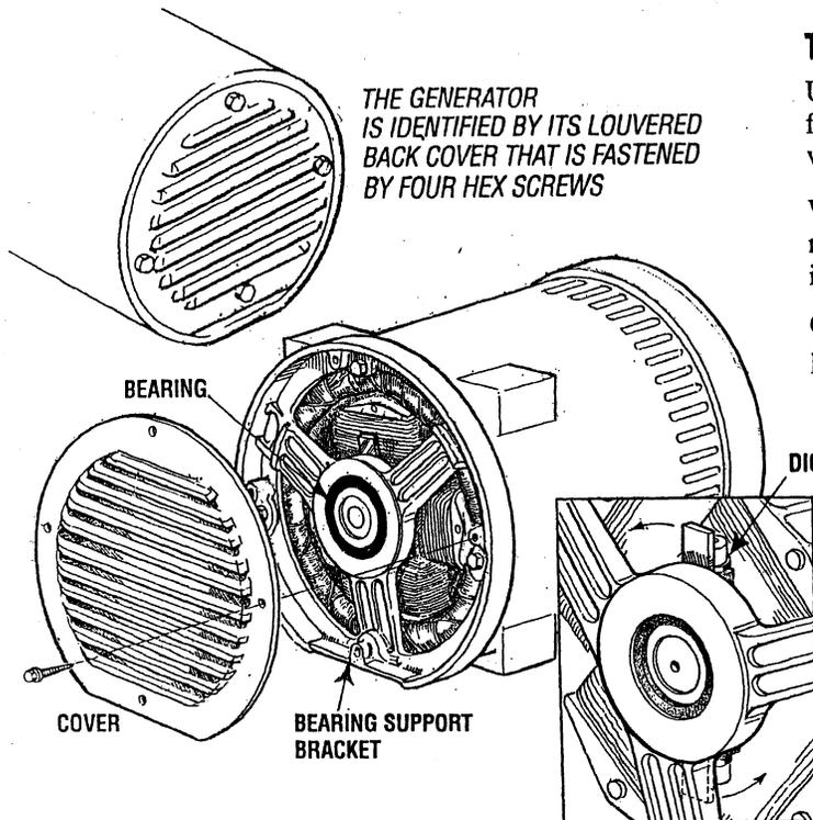
THE GENERATOR IS IDENTIFIED BY ITS LOUVERED BACK COVER THAT IS FASTENED BY FOUR HEX SCREWS
