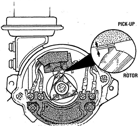
Adjust the point gap of the pick-up assembly between the rotor and the pick-up.
