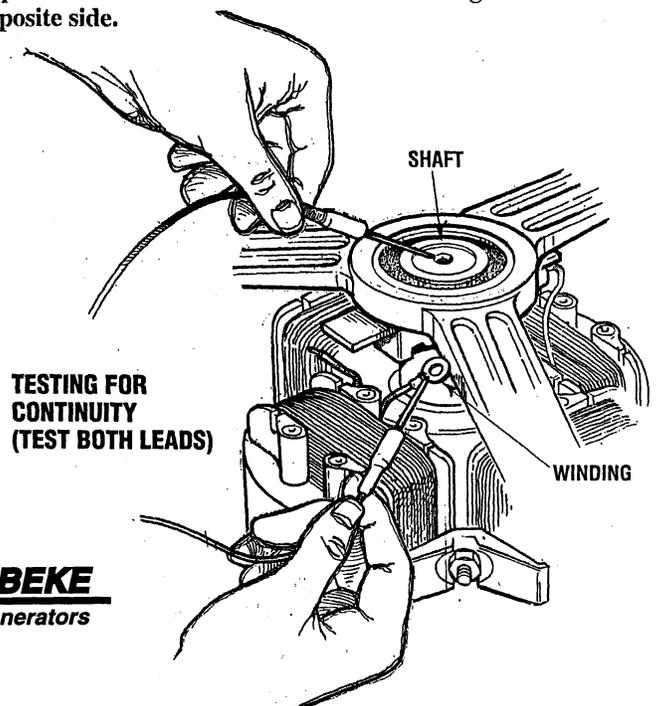
TESTING FOR CONTINUITY (TEST BOTH LEADS)
