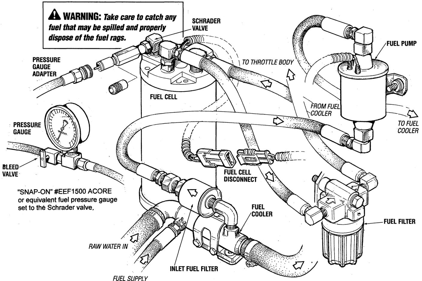
"SNAP-ON" #EEF1500 A CORE or equivalent fuel pressure gauge set to the Schrader valve.
