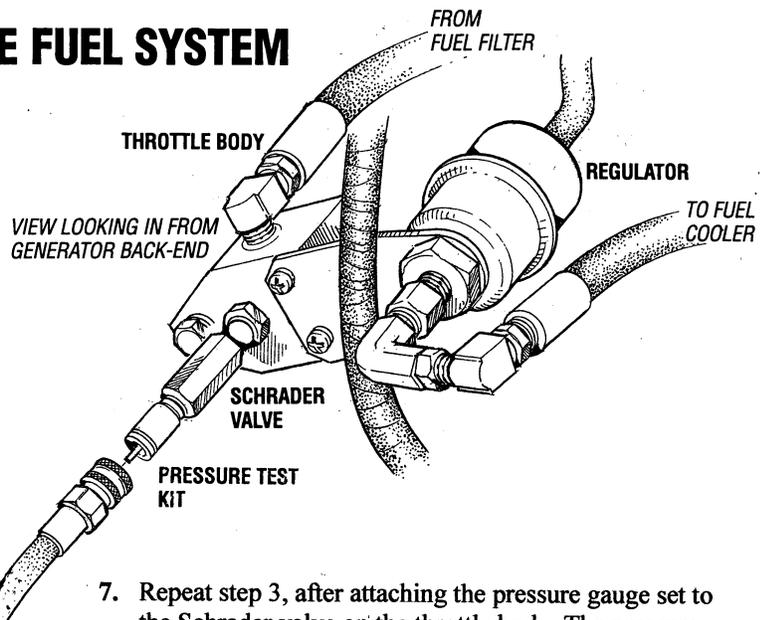
7. Repeat step 3, after attaching the pressure gauge set to the Schrader valve on the throttle body. The pressure should be 40 psi after purging all the air.
