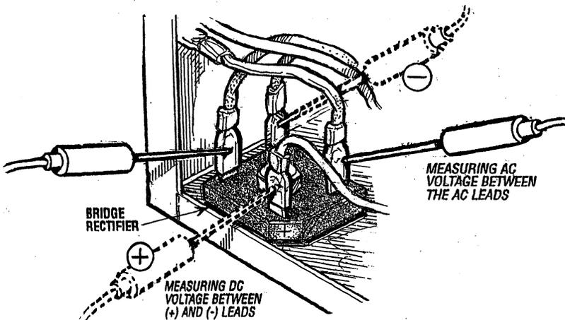
Normal DC voltage running out of the rectifier (in volts DC) is measured across the two DC connections of the bridge rectifier, that is + and - as illustrated.
