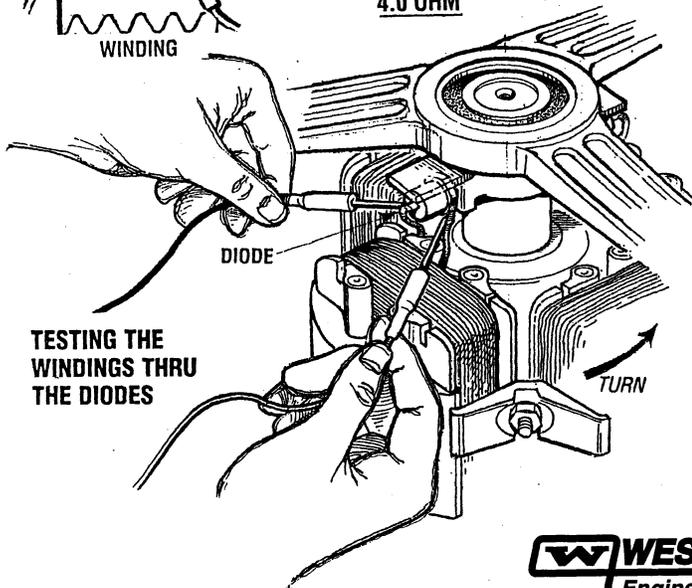
TESTING THE WINDINGS THRU THE DIODES
