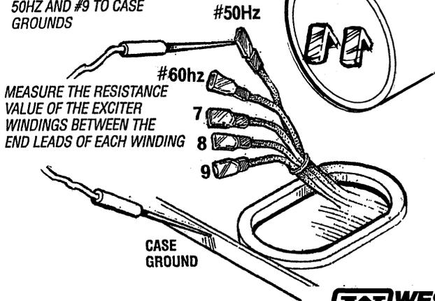
MEASURE THE RESISTANCE VALUE OF THE EXCITER WINDINGS BETWEEN THE END LEADS OF EACH WINDING
