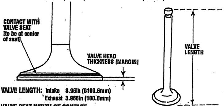
**VALVE LENGTH:** Intake 3.96in (100.6mm)
