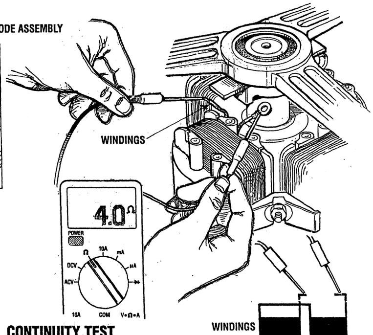
Testing the generator can be accomplished without removing the bearing support bracket. Simply turn the armature to allow access for the testing as shown.
