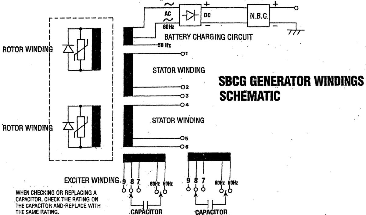
WHEN CHECKING OR REPLACING A CAPACITOR, CHECK THE RATING ON THE CAPACITOR AND REPLACE WITH THE SAME RATING.
