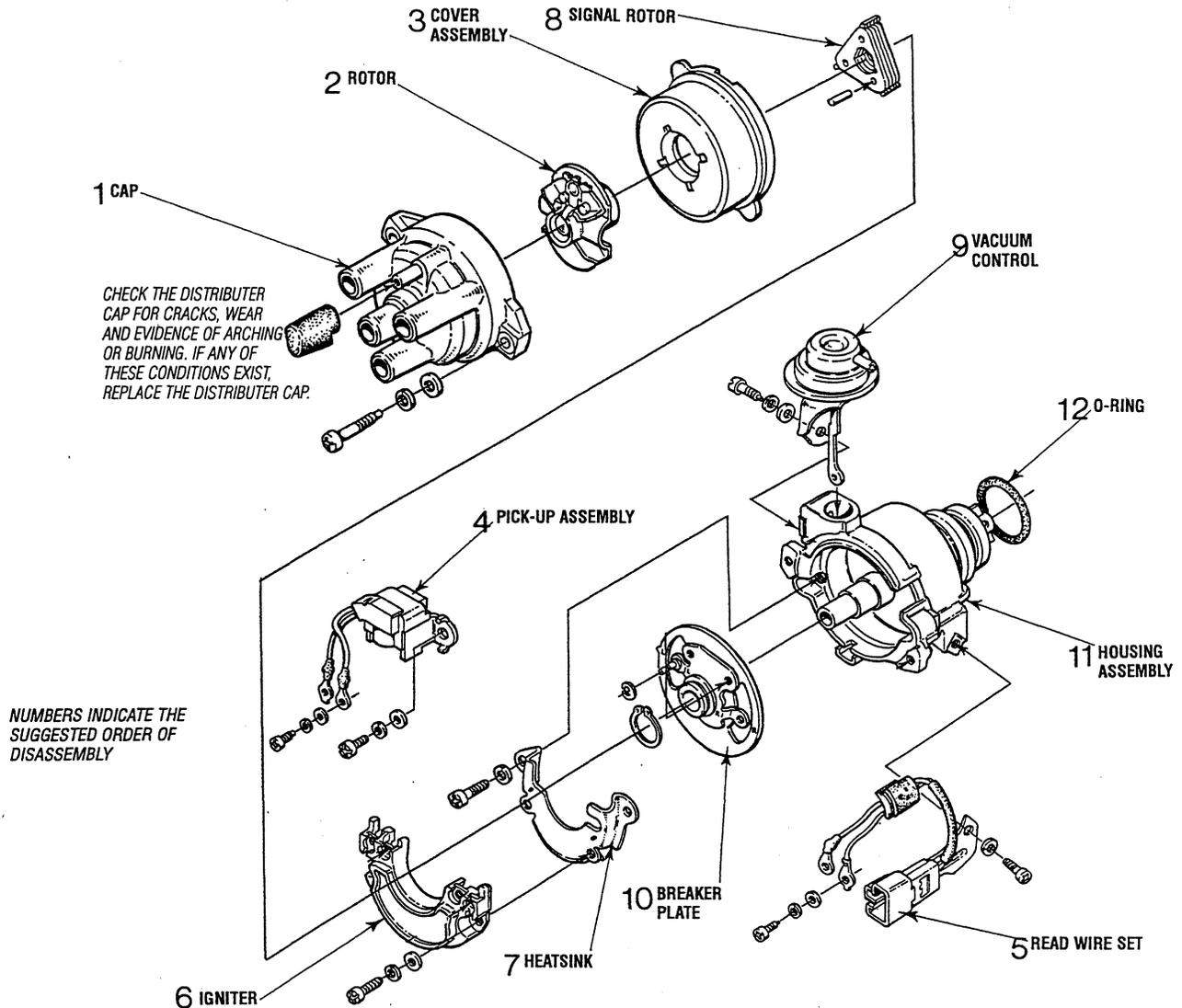
**NOTE:** When engaging the Distributer Drive into the Camshaft match the markings for correct engagement.
