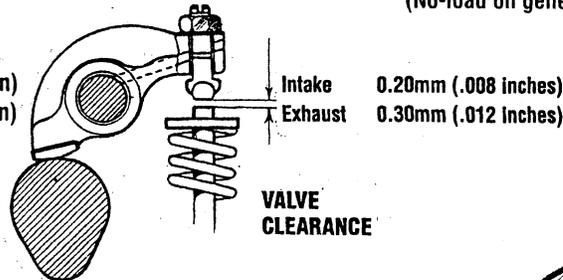
Rotate the crankshaft 120 degrees to position the piston in cylinder #3 at TDC of its compression stroke and adjust this cylinder's exhaust and intake valves. Rotate the crankshaft another 120 degrees to position the piston in cylinder #2 at TDC of its compression stroke and adjust this cylinder's intake and exhaust valves.
