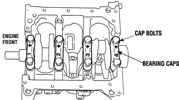
2. Install the bearing cap paying careful attention to the cap number and the arrow mark. Apply oil to the bolt threads.
