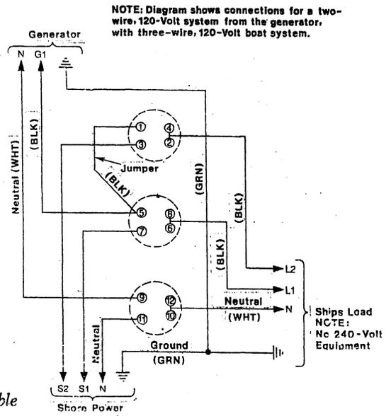
**NOTE:** Diagram shows connections for a two-wire, 120-Volt system from the generator, with three-wire, 120-Volt boat system.
