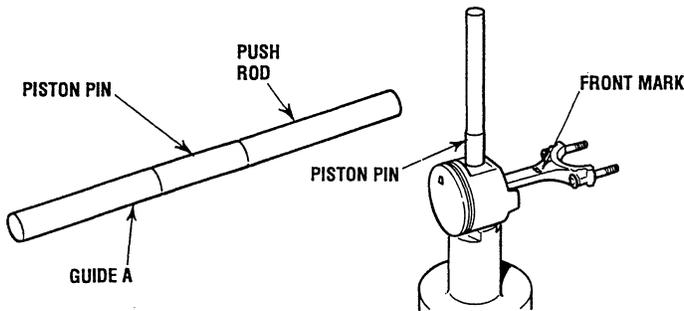
Set up the piston and connecting rod on the piston pin setting base. Make sure that the front marks are facing up. Apply engine oil to the outer circumference of the piston pin and insert the pin, Guide A and the push rod (assembled) into the piston and connecting rod.
