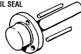
**PIN** *For supporting the sprocket when the camshaft sprocket is loosened or tightened.*
